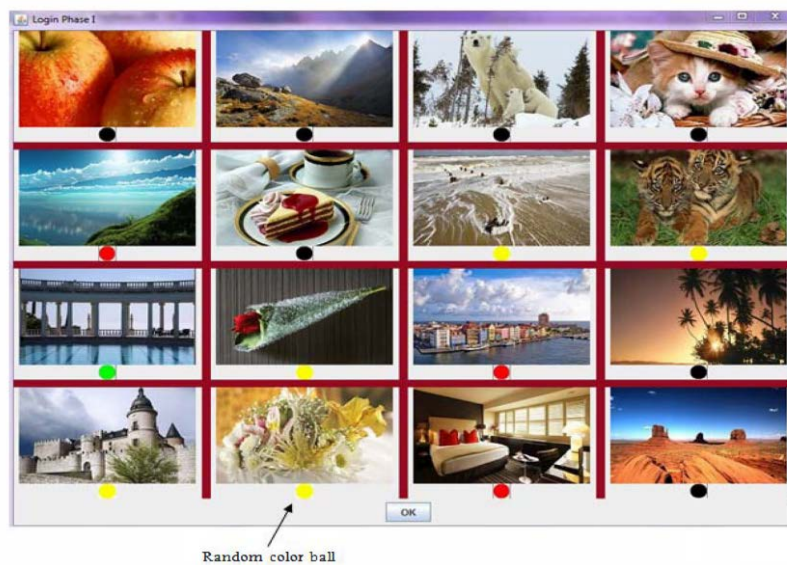
Fig. 18: The first authentication phase, 4x4 grid and associated colour balls
